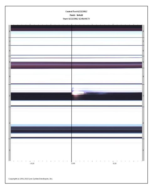
Figure 17: Example of Zero Gun Test result with an electronic gun
